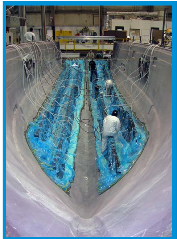
Primary PVC foam cored longitudinal stringers are infused into the hull.
