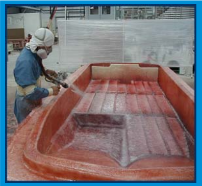
Encapsulating custom-made foam cores with fiberglass and AOC resin is part of Sundance's process for manufacturing an integral hull in a single cure cycle.
