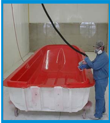
Vibrin® gel coats are applied in Sundance's state-of-the-art production facility and produce state-of-the-art surfaces.
