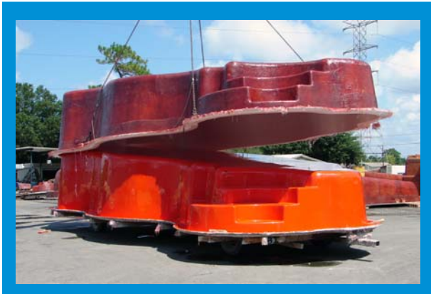
A Blue Hawaiian Fiberglass product is pulled from the mold.
