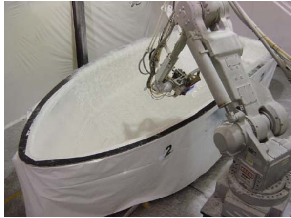
Hydropel® R580-CUC low-profile resin allows Sea Ray to use RIMFIRE® preforms without having to use a veil.
