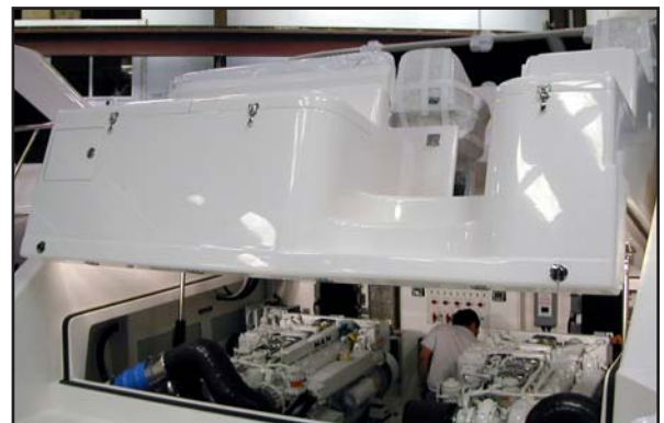
Cabo's unique hydraulic-lift helm deck on Express models provide easy access to the engine (top photo: curing in the shop; bottom photo: installed and in use).
