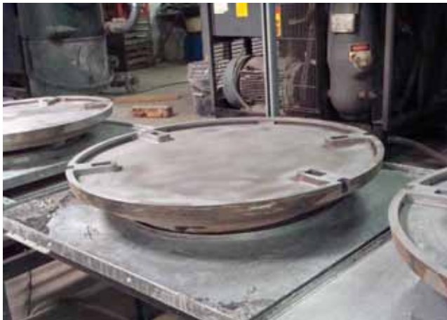
Production starts by grit-blasting a cast iron "dish."
