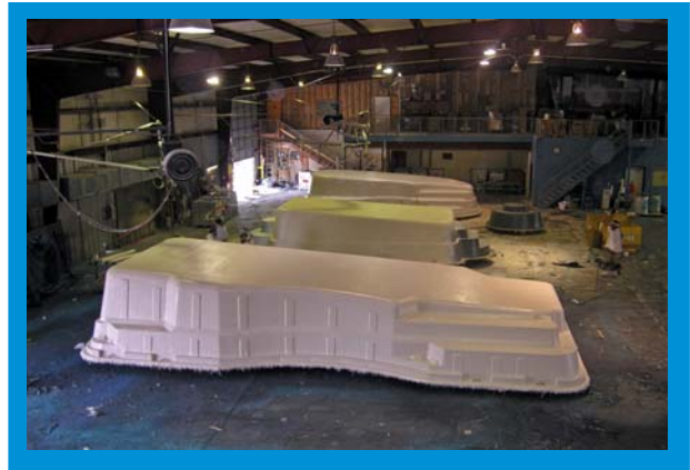
Good fiber wetting with the AOC vinyl ester facilitates the application of a barrier coat that protects the gel coat surface from blister-causing osmosis
