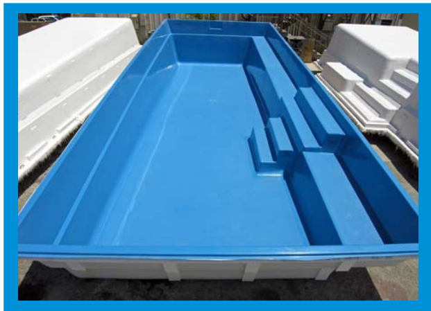
A finished Grand Elegance Style model is out of the mold in the Leisure Pools manufacturing facility.
