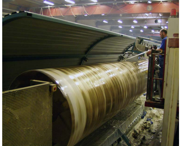
The stack liners were manufactured using Tunetanken's cutting-edge winding technology.
