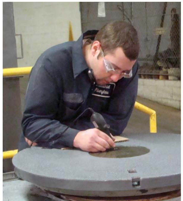
A serial number is engraved into each part before shipping.
