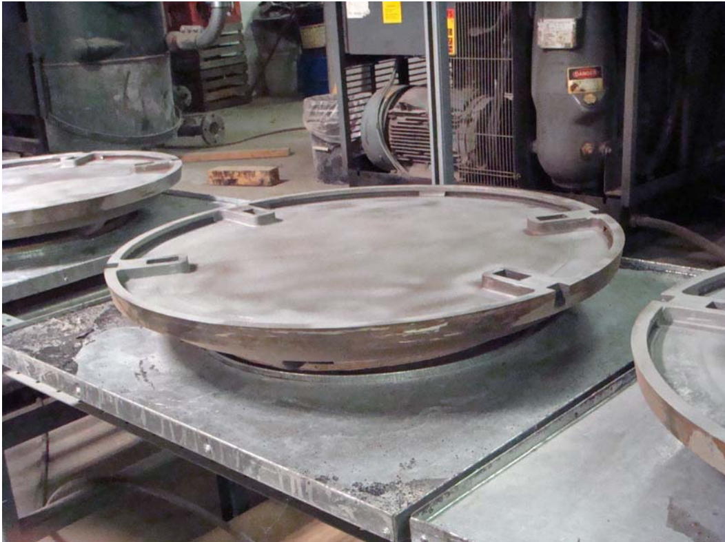
Production starts by grit-blasting a cast iron "dish."
