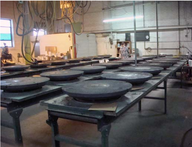
The composite cures into a high-strength, thermally-insulating layer.
