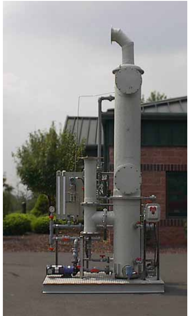
Because it is made with Vipel® K022-C vinyl ester, this emergency scrubber is designed to resist the corrosive effects of ammonia if ever called into action.
