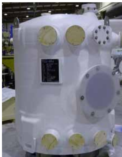
RL Industries use Vipel® F010 Vipel F010 bisphenol A epoxy vinyl ester resin to manufacturer dual laminate tanks for the semi-conductor industry
