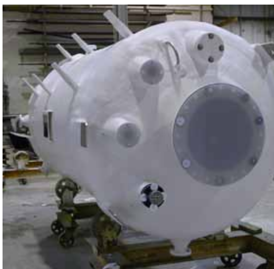
RL Industries use Vipel® F010 Vipel F010 bisphenol A epoxy vinyl ester resin to manufacturer dual laminate tanks for the semi-conductor industry
