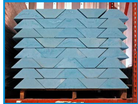
Pre-cut foam was integrated into the circumference of each section to help form exterior structural ribs that help support the liner.
