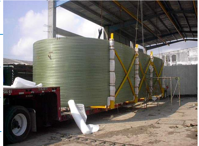
To reduce shipping costs, wall ring sections were obliterated into narrow profiles at the composite fabrication plant.
