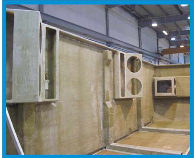
Some ventilation system housings are designed to be intergrally molded into the nacelle interior.
