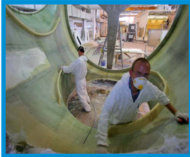
Markos workers finish the interior of a 9-meter long nacelle.
