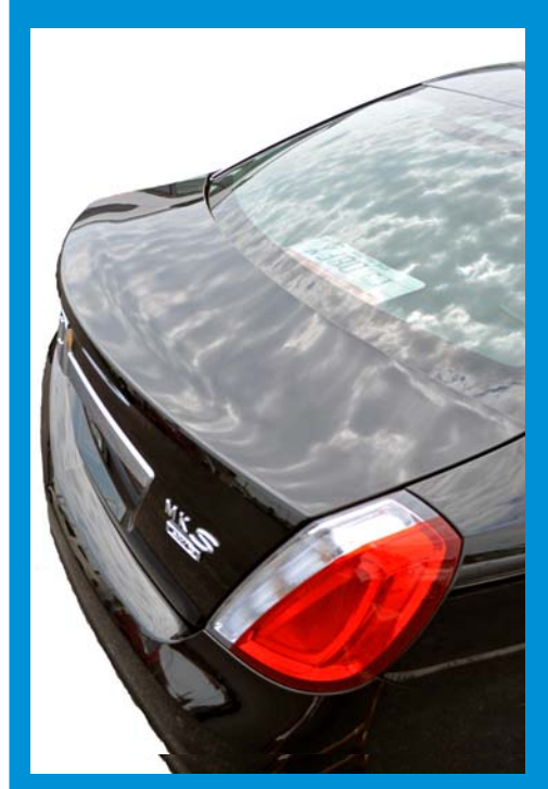
Continental Structural Plastics worked with AOC to develop a sheet molding composite (SMC) that offers superior edge-pop resistance through the paint process.
