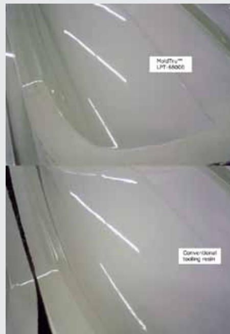
Surface comparison of covers made with MoldTru™ resin and conventional tooling resin
