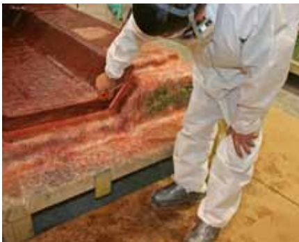
Rolling out a tight radius
