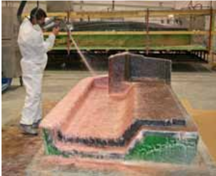
Application of the first bulk layer
