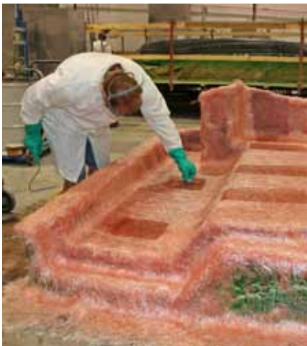
Measuring the first layer thickness
