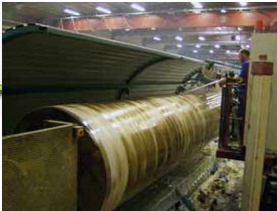
The liners are made from filament wound sections.
