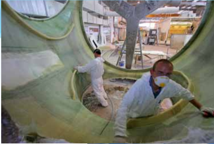
Markos workers finish the interior of a nacelle.
