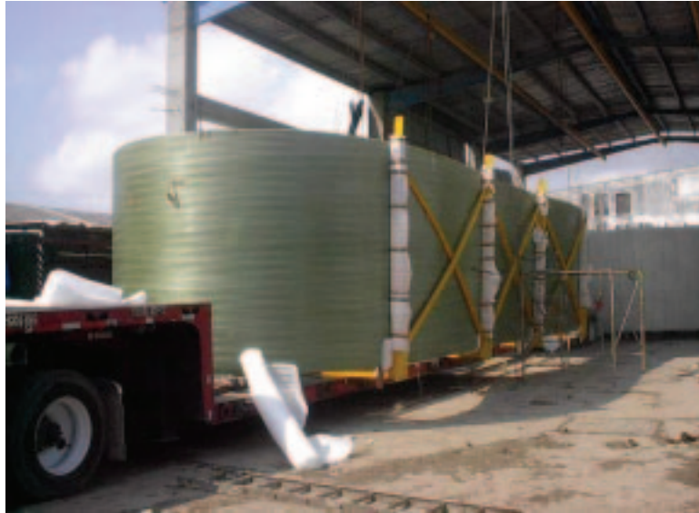
Figure 2. Composite tank sections are oblated to reduce their footprint for shipping.
