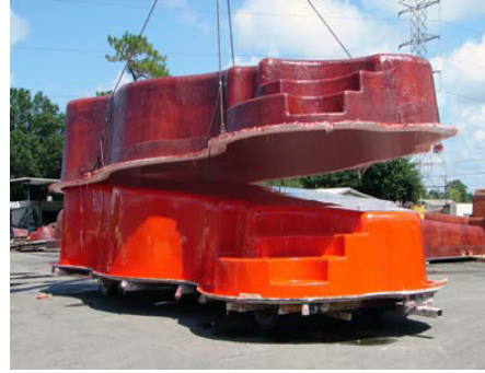
A Blue Hawaiian Fiberglass product is pulled from the mold.
