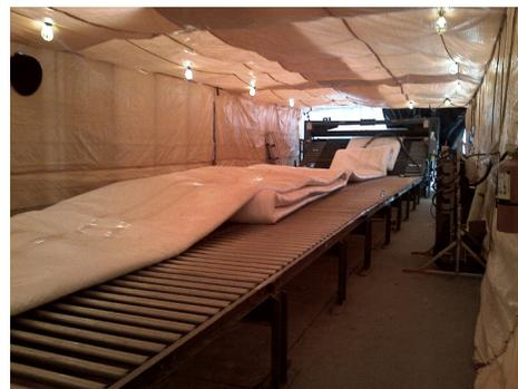
Onsite roller bed and liner are prepared for resin impregnation.
