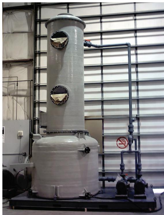
*Because it is made with Vipel® K022-C vinyl ester, this emergency scrubber is designed to resist the corrosive effects of ammonia if ever called into action.*
