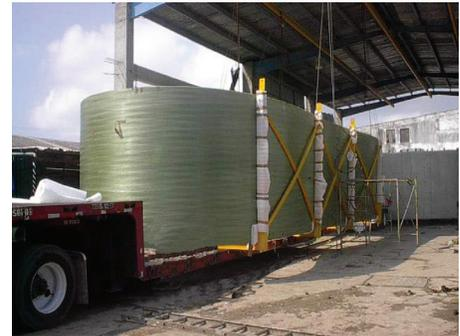
To reduce shipping costs, wall ring sections were oblated into narrow profiles at the composite fabrication plant.
