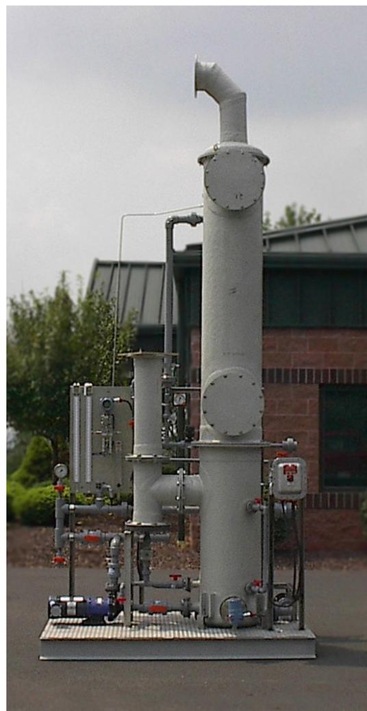
*Because it is made with Vipel® K022-C vinyl ester, this emergency scrubber is designed to resist the corrosive effects of ammonia if ever called into action.*
