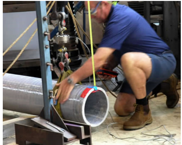
This 9.5-meter power pole from A.C. Whalan Composites was designed for installations with limited access. The two-piece section can be assembled on site without the expense of heavy lift cranes.
