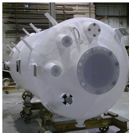
*Because it is made with Vipel® K022-C vinyl ester, this emergency scrubber is designed to resist the corrosive effects of ammonia if ever called into action.*
