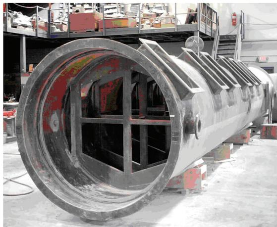
To remove process-generated pollutants, a large steel producer specified three tray towers fabricated of fiber-reinforced polymer composite. But after 15 years, the towers started “ imploding ” even though they had been repaired numerous times. To solve their problem, engineers asked Heil® Process Equipment to replace the failing equipment with an improved tray tower manufactured with Vipel vinyl ester from AOC.
