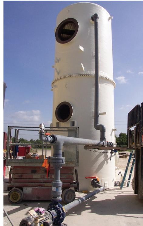
Corrosion-resistant Vipel K022-C is used to fabricate composite equipment that is essential to controlling odors from a new million gallon per day wastewater treatment facility. Belco Manufacturing, Belton, TX, USA, uses Vipel K022-C vinyl ester to filament wind cylindrical components and open mold elbows and flanges. Scrubber systems are
