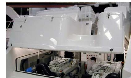
*Cabo's unique hydraulic-lift helm deck on Express models provide easy access to the engine (top photo: curing in the shop; bottom photo: installed and in use).*
