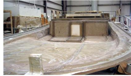
*The surface of the deck-in-progress is mechanically ground to ensure good adhesion of the next layer of composite laminate.*
