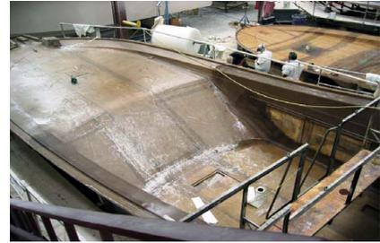
*Cabo Yacht decks are handcrafted of fiberglass roll goods and AOC resin by highly skilled workmen.*
