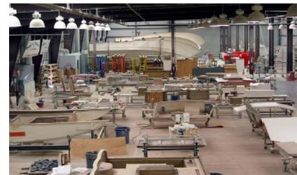
*In Cabo Yachts' clean, modern facility, AOC resin is used to mold decks, flying bridges, and a host of smaller components.*
