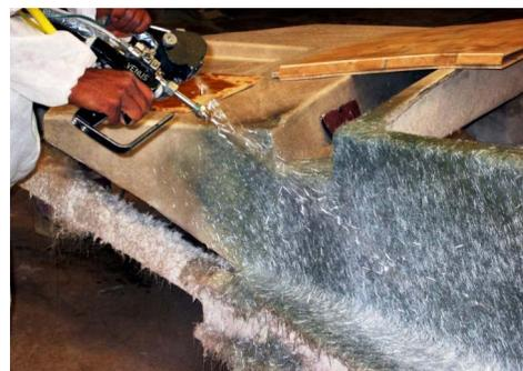
*To effectively get around the tight corners of complex inner liners, Oskinning out is accomplished with a chopper gun.*
