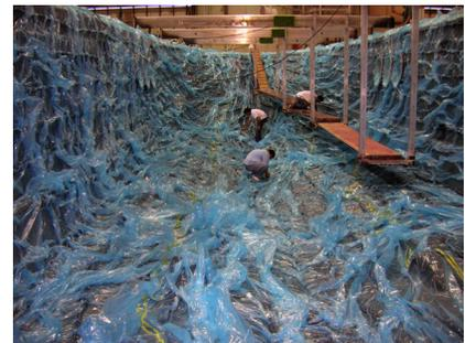
*During resin infusion, 29 inches vacuum of mercury is pulled under a polymer film.*
