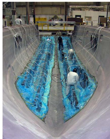
*Primary PVC foam cored longitudinal stringers are infused into the hull.*
