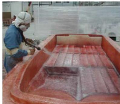
*Encapsulating custom-made foam cores with fiberglass and AOC resin is part of Sundance's process for manufacturing an integral hull in a single cure cycle.*
