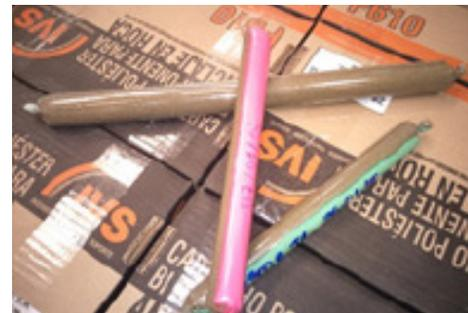
*The two-component polyester resin cartridges are critical to anchoring rock bolts to the surrounding strata in underground mines.*
