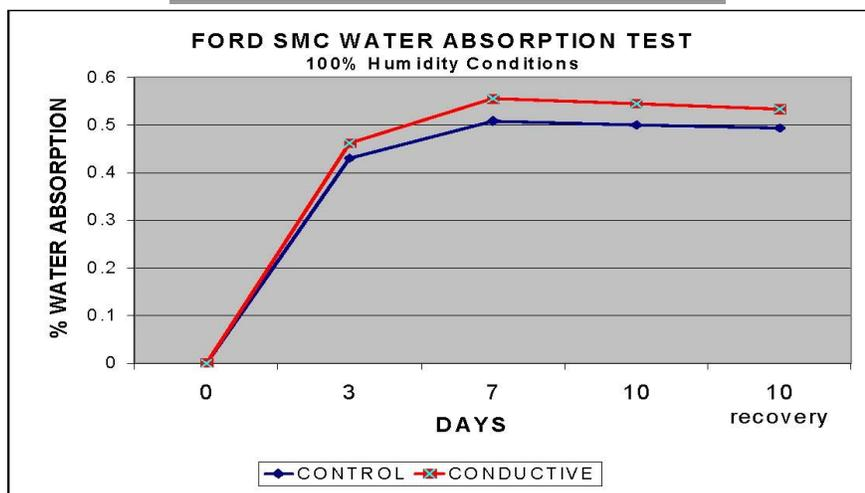
Figure 2. Ford SMC Water Absorption Test
