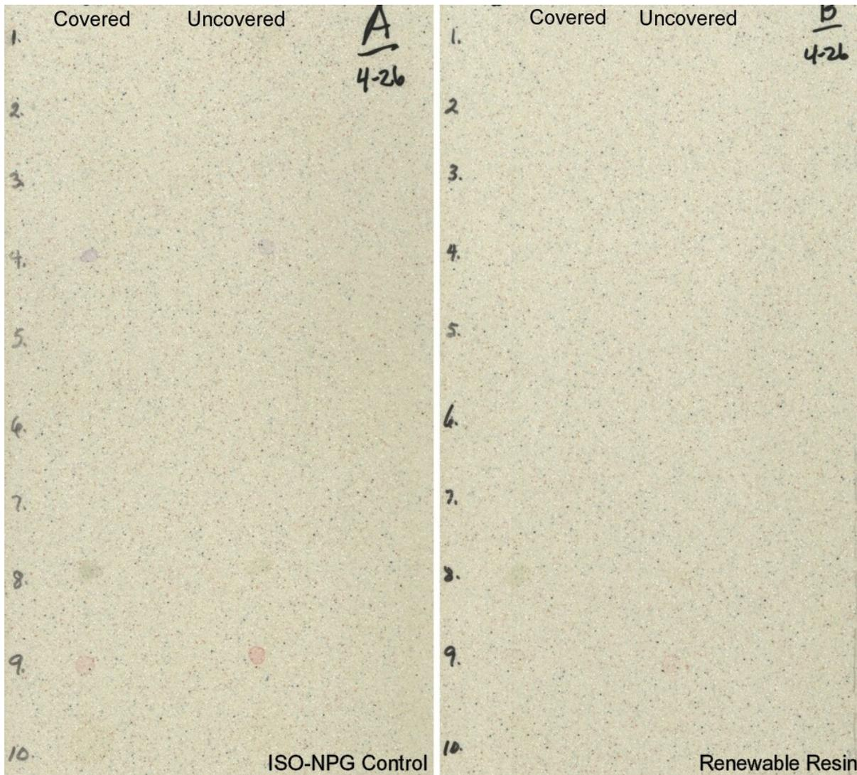
**Figure 4:** ANSI/ICPA SS-1-2001 Stain resistance test specimen comparison of the renewable-derived solid surface resin (right) and the industry standard ISO-NPG resin (left). Stain tests as follows: (1) black crayon; (2) black liquid shoe polish; (3) blue washable ink; (4) gentian violet solution; (5) beet juice; (6) grape juice; (7) lipstick; (8) black hair dye; (9) mercurochrome solution, 2%; (10) wet tea bag.
