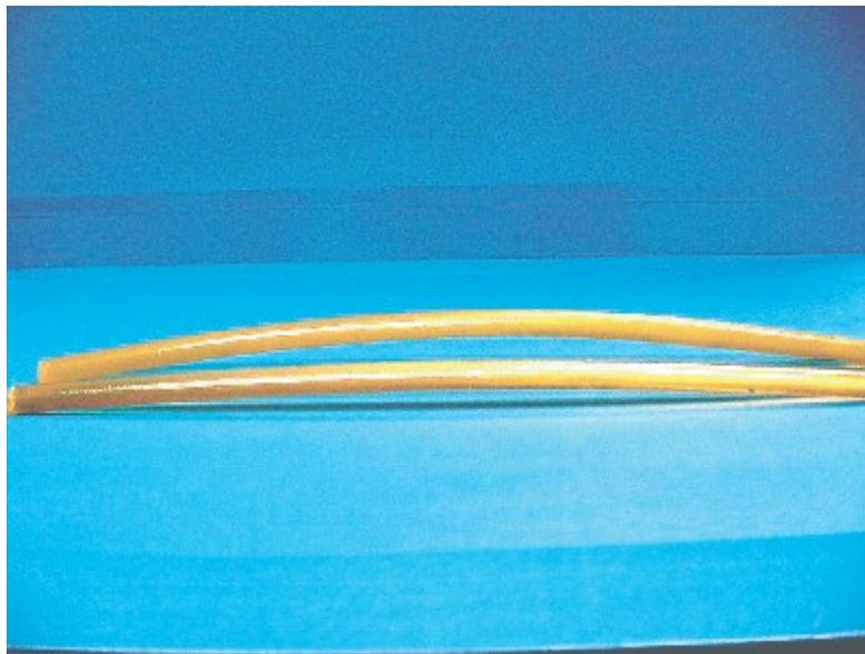
Figure 7. The photo above demonstrates the improved HDT of the new polymer without the addition of filler. The front test bar is the new polymer. The specimen in the background is an example of traditional resin systems that have lower HDT temperatures.
