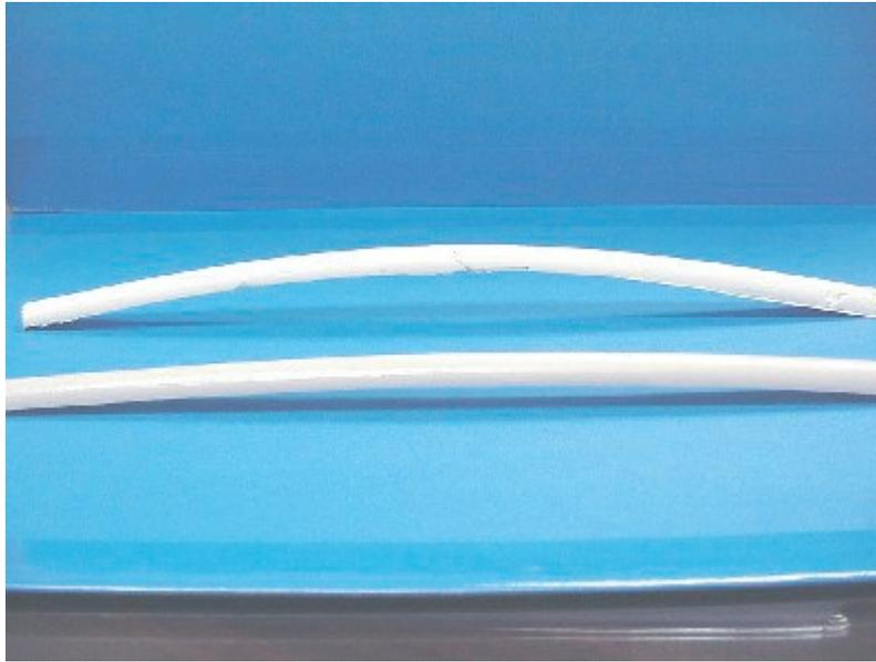
Figure 6. The photo above demonstrates the improved Heat Distortion Temperature of the new polymer filled. The front specimen is the new polyester. The specimen in the background is a sample from the traditional polyester resin system.
